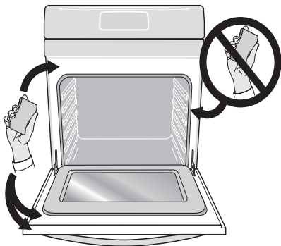
Figure 19: Clean around oven door gasket
